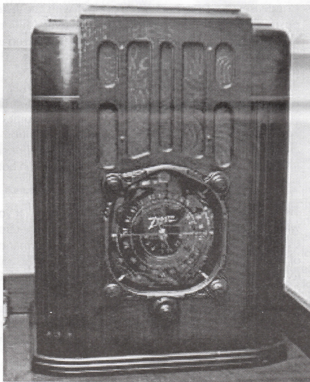
A Zenith 10S130. Just from the model number we can deduce ten tubes, 1937 model year, 110 VAC, three bands, high-end tabletop.
